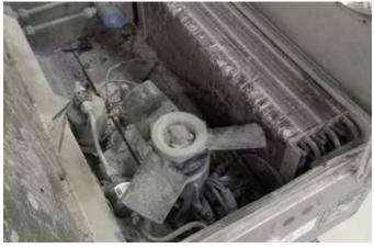
A unit that has been returned for overhaul, after enduring 7+ years of operation on a blasthole drill.
